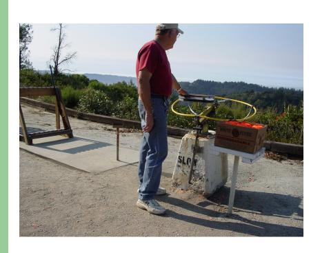
With your foot well away from the foot pedal release, rotate the throwing arm into the cocked position.
