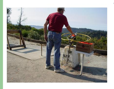
Load a biodegradable bird onto the cocked throwing arm, between the rubber bumper and the black line on the throwing arm. This is the only acceptable area on the throwing arm to place your bird.
